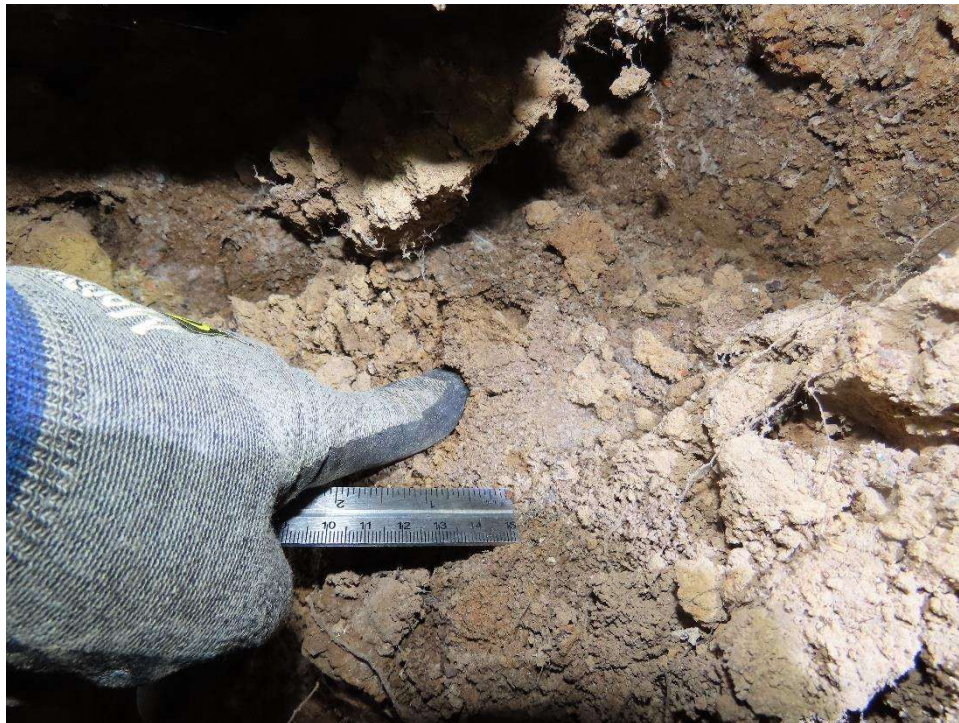
Photo 15: The soil yielded to finger pressure.
