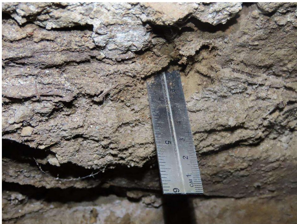
Photo 16: A metal ruler was easily inserted into the supporting soil.
